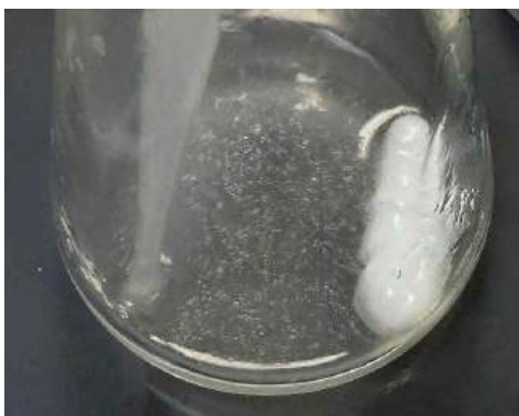
Figure 2. Finished silica solution with a pipette tip on the left and a magnetic stirrer on the right. Image taken by student researcher, 2025.
